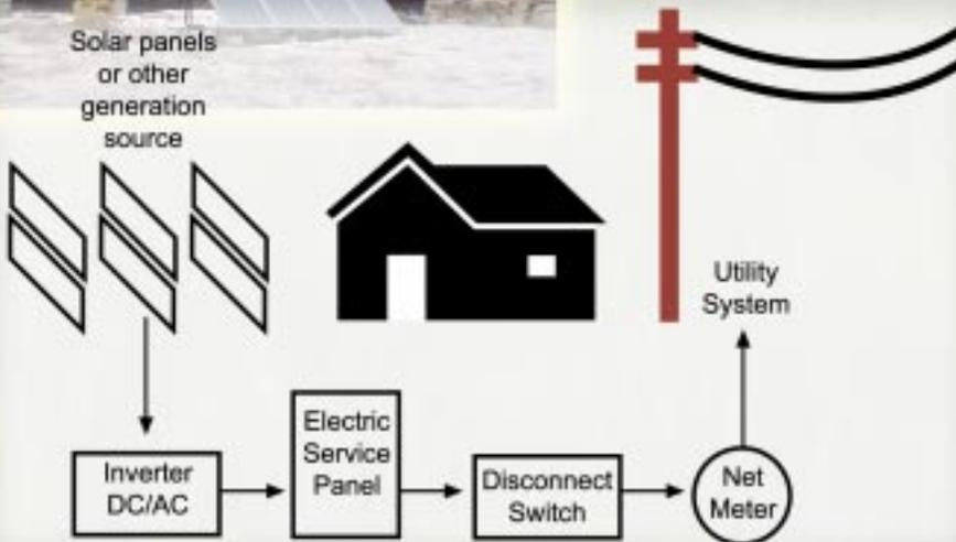
The diagram to the left outlines the essentials of a net metering system. In most locations within the Valley, solar panels offer the most promise for consumer generation. With photo-voltaic generation systems, an inverter converts DC power to AC power. Power feeds into the member's electric service panel. A disconnect switch protects both the homeowner and utility workers. The meter records both member use and member generation.
